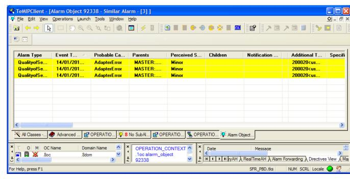
Figure 18: Display similar alarms of a sub-alarm
