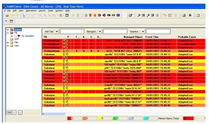
Figure 3: Filter pattern [No SubAlarm] deactivated: 20 alarms displayed
