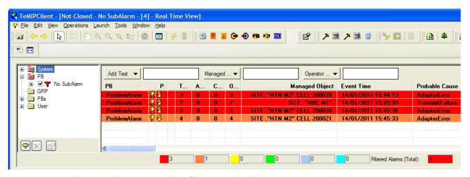
Figure 4: Filter pattern [No SubAlarm] activated: 4 alarms displayed vs. 20
