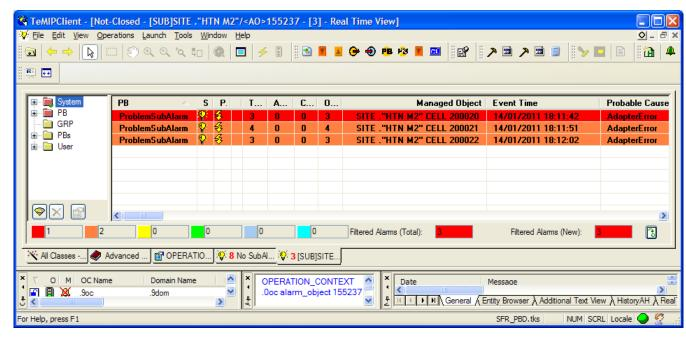
Figure 6: ProblemSubAlarms are displayed by the drill down button
