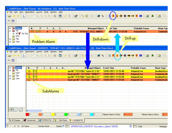
Figure 20: GSM Ericsson Cell Down Problem Alarm display
